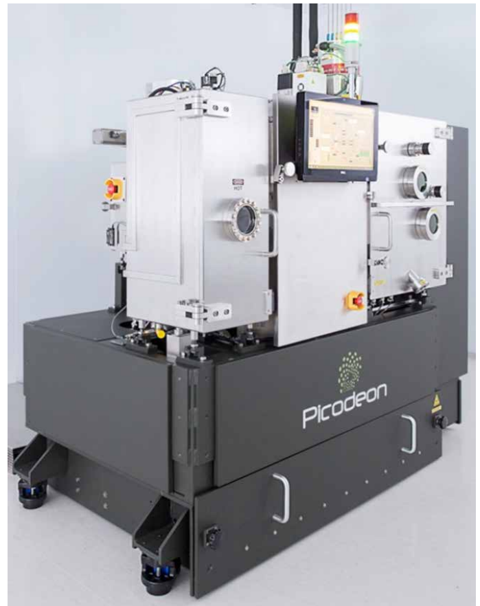
Picodeon Series4 semi-industrial automated PLD system
